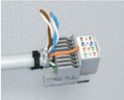
Device connection – cable sorting Attach the individual wires according to the connection table and fix the using the contacting terminal.
