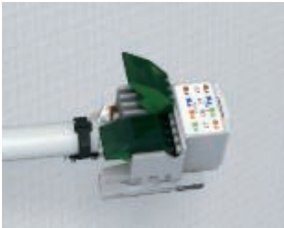
Device connection – cable attachment Place the contacting bracket on the connection module and lock it in place. In the shielded version, the shield housing must also be attached.
