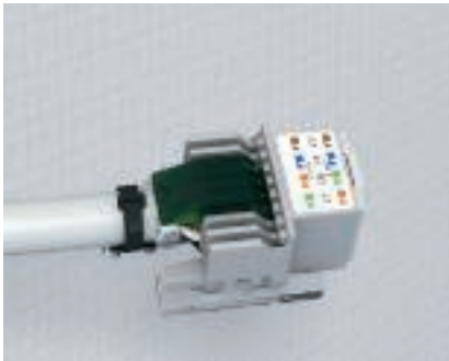
Device connection as RJ11 telephone socket When used as a telephone connection box, wire only the inner connection points. The reducing frame (type DMZ-RR/RJ11) prevents unintentional insertion of RJ45 connectors into the telephone socket.
