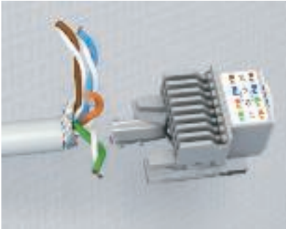
Device connection – cable preparation Remove the outer jacket of the data technology cable and, if necessary, the insulation to a length of 50 mm.
